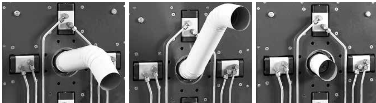
New programs are easily added to the machine, creating product such as a downspout with an "S" curve in one single piece.
