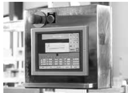
Changing the elbow angle and pipe length requires no manual settings – the machine is controlled through an easy-to-use user interface.
